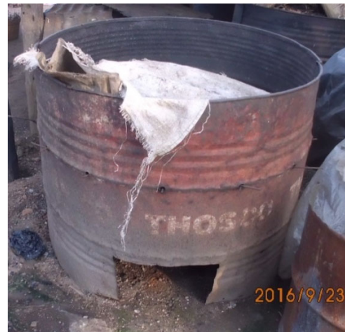
Figure 3. Traditional kiln made with three connected sections of open drums at Grand-Lahou
