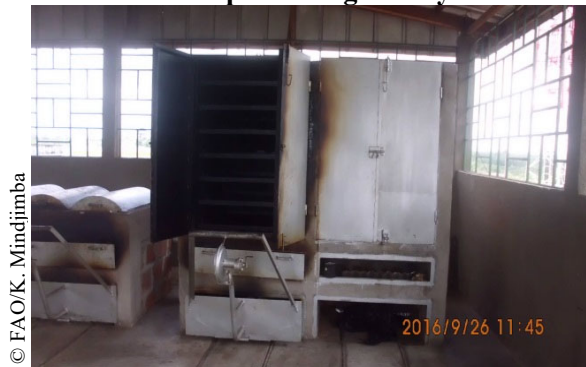
Figure 9. FTT Altona kiln with two compartments at the Guessabo processing facility
