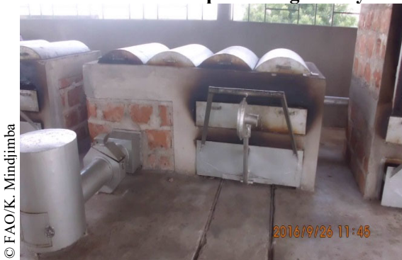
Figure 8. FTT Banda kiln with a smoke filter at the Guessabo processing facility
